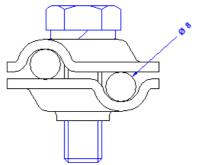
Suitable as well for use as T-, parallel and cross-clamp.
