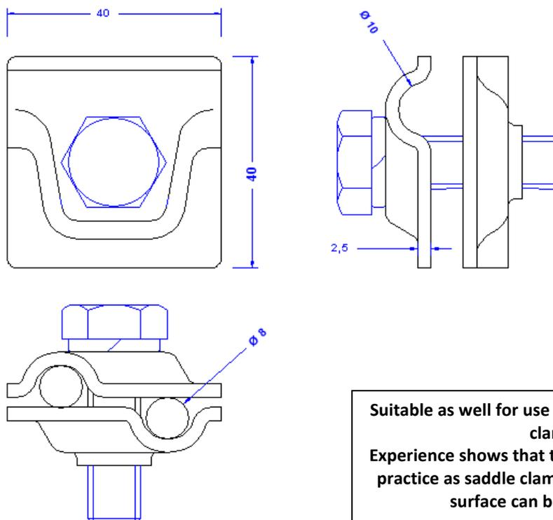
**Suitable as well for use as T-, parallel and cross-clamp. Experience shows that this clamp is also used in practice as saddle clamp if a sufficient contact surface can be guaranteed.**
