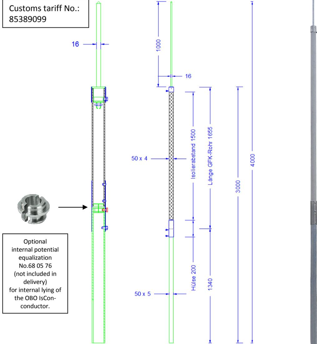
Optional internal potential equalization No.68 05 76 (not included in delivery) for internal lying of the OBO IsCon-conductor.
